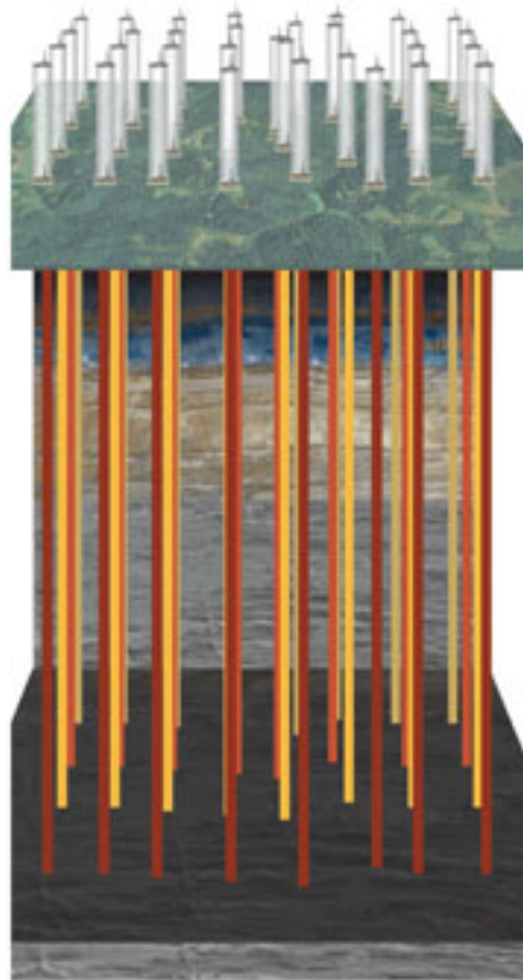
Traditional Vertical Well Spacing: 32 Separate Padsites Needed For 32 Wells.
